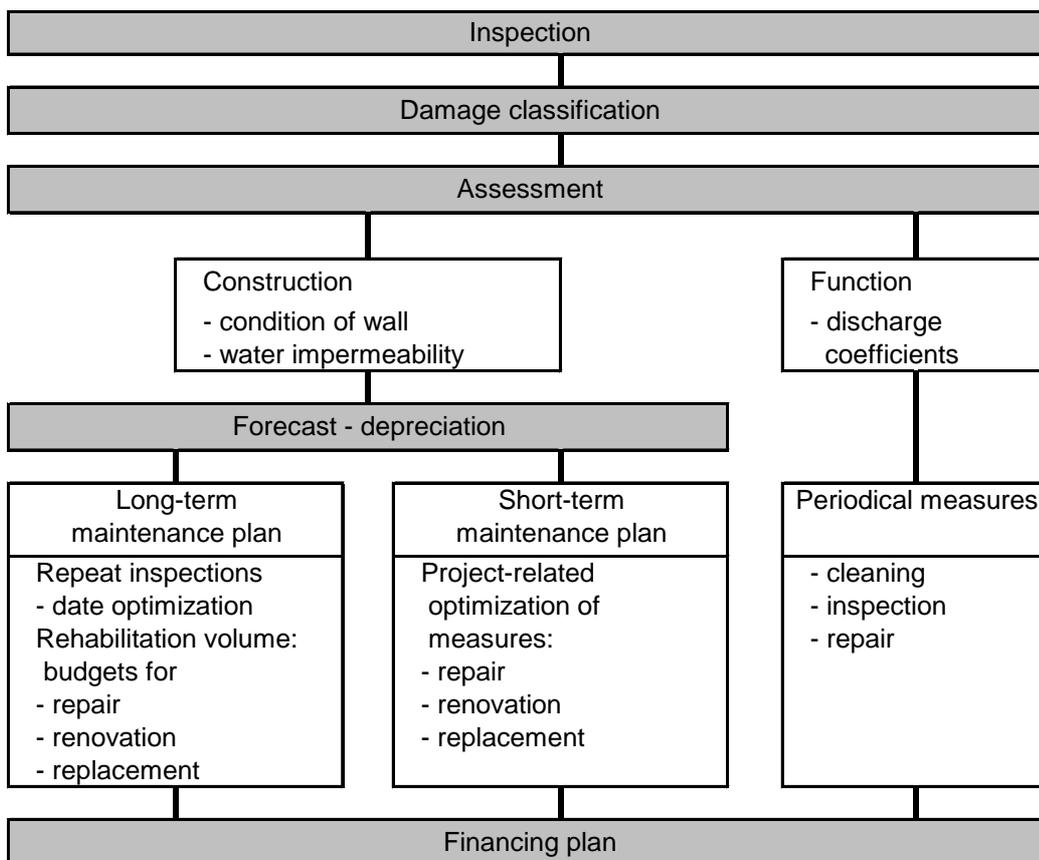
Diagram 2: Flow chart of a modern sewer management system according to [7]
