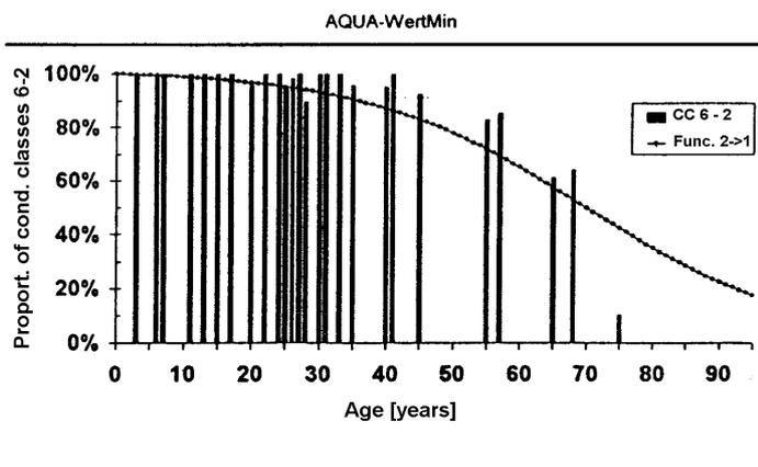
Diagram 4: Condition transition function from class 1 to class 2
