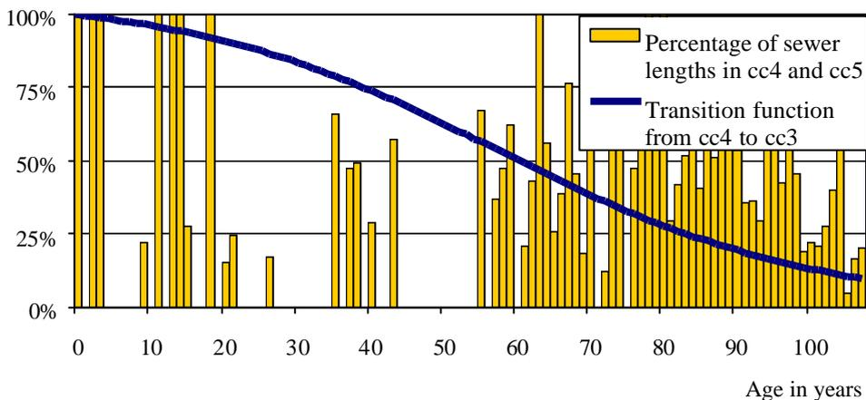
**Figure 2:** Calibrated transition function from cc4 to cc3, good to not so good
