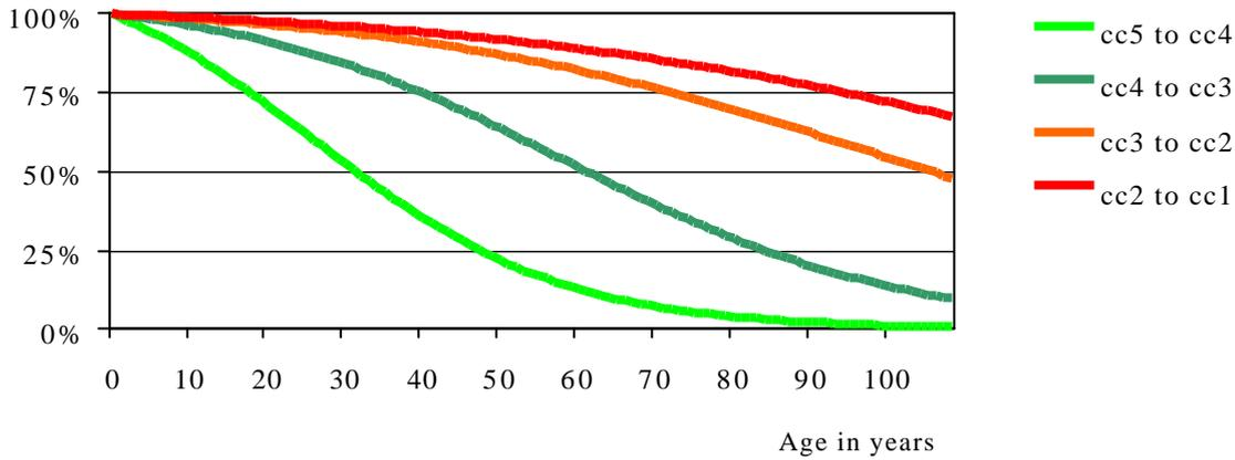
**Figure 3:** Transition functions for the Dresden sewer sample
